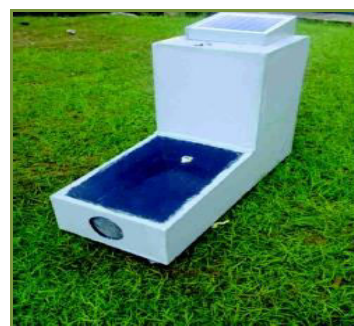
Figure.27 Indirect forced convection solar dryer to dry cassava chips
