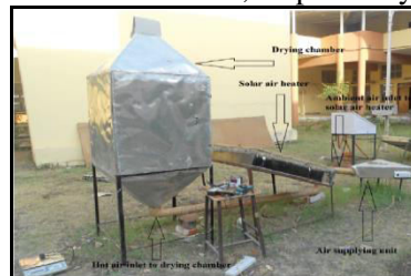
Figure.30 Indirect solar dryer for fenugreek drying
