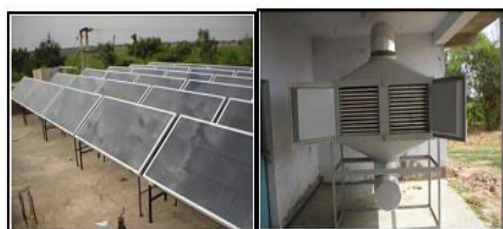
Figure.20 Packed bed solar air heaters and drying chamber of indirect forced convection solar cabinet dryer with LPG back up for tomato drying
