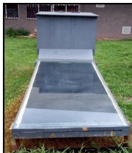
Figure.32 Indirect forced convection solar dryer for cocoa beans
