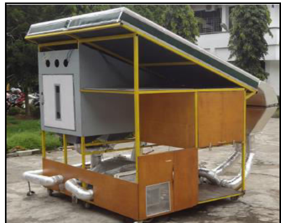
Figure.12 Solar-assisted heat pump dryer (SAHPD)
