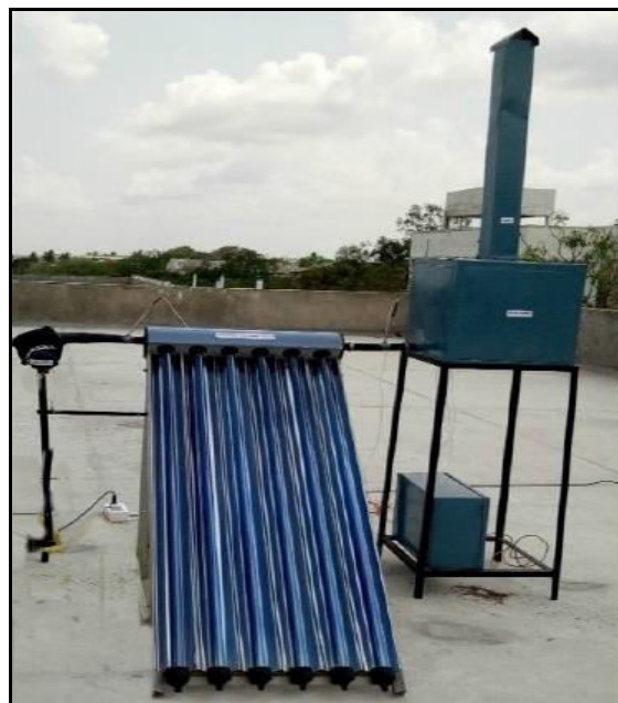
Figure.35 Evacuated tube collector based forced convection indirect solar dryer
