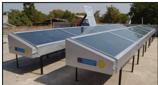
Figure.23 Indirect type solar forced circulation tunnel dryer for amla
