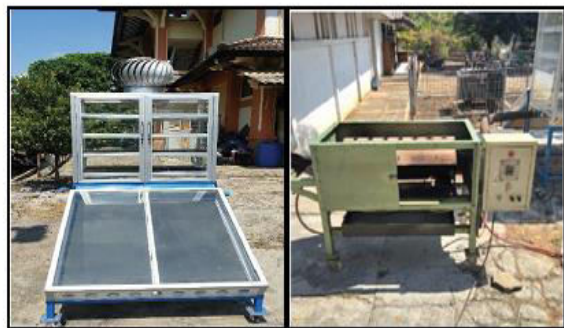
Figure.38 Hybrid solar dryer with blower-burner unit
