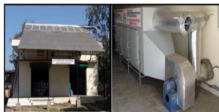
Figure.21 Roof integrated glazed and unglazed solar dryer for ayurvedic medicinal powder and herbs oyster mushroom
