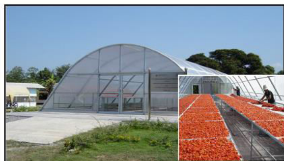
Figure.26 Large-scale solar greenhouse dryer with LPG burner
