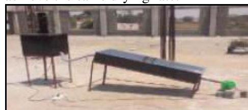
Figure.28 Laboratory scale forced convection solar dryer for drying Amla
