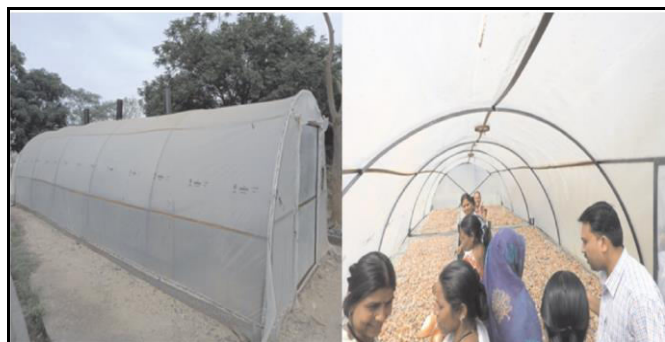
Figure.39 Solar tunnel dryer for keshuda drying
